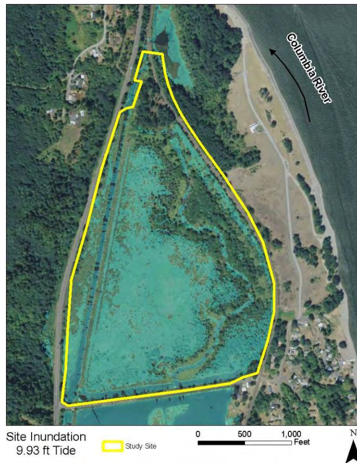
Figure 24. Approximate inundation at 9.93 ft, the highest water level observed at the C2 station for the comparable monitoring period for the three stations (2009 aerial photograph).
