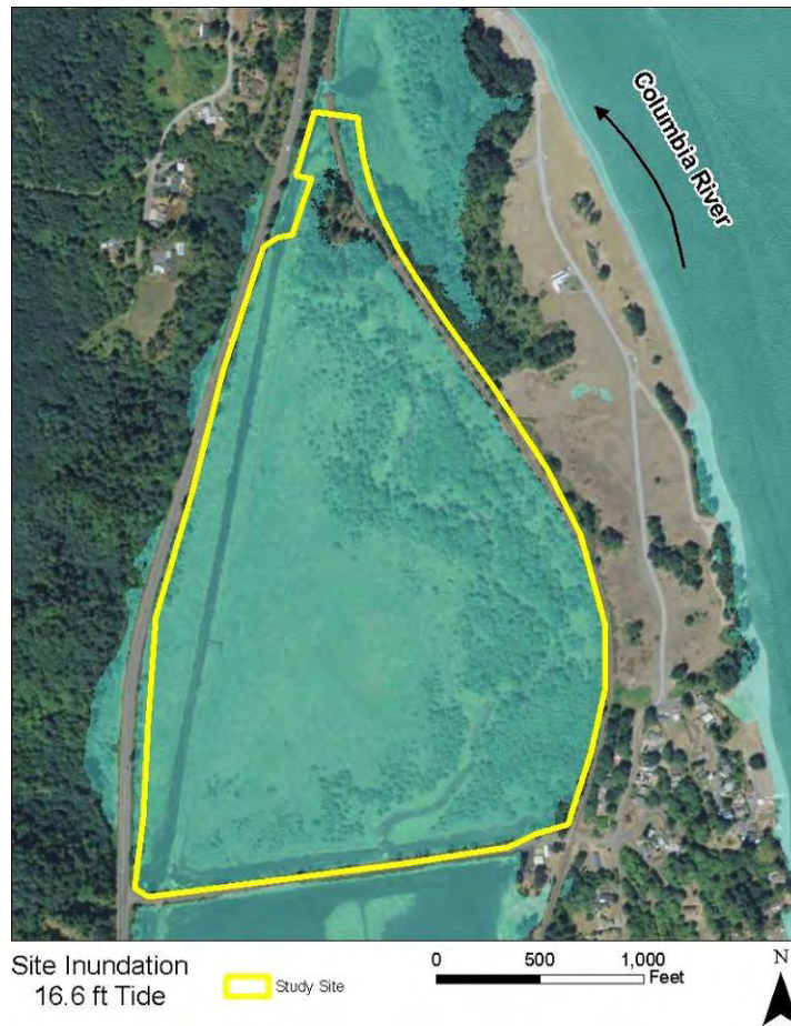
Figure 22. Approximate inundation at a water surface elevation of 16.6 ft, the highest water level observed at the C2 station during the monitoring period (2009 aerial photograph).
