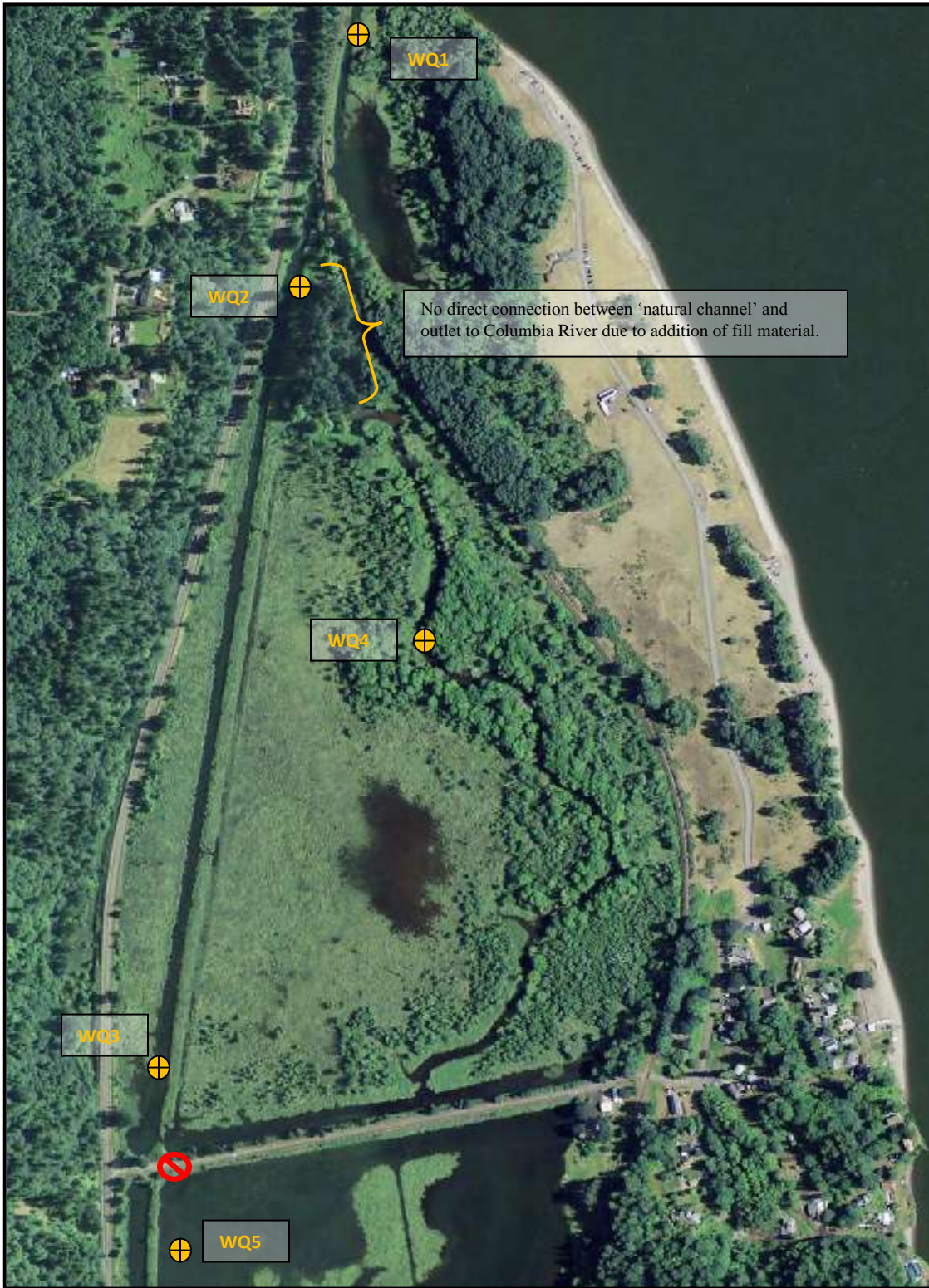
Figure 2. Aerial Photograph of Carr Slough Showing Current Site Conditions. Potential water quality sampling sites are noted in orange. The current tide gated culvert connecting Carr Slough to the adjacent parcel is indicated in red.
