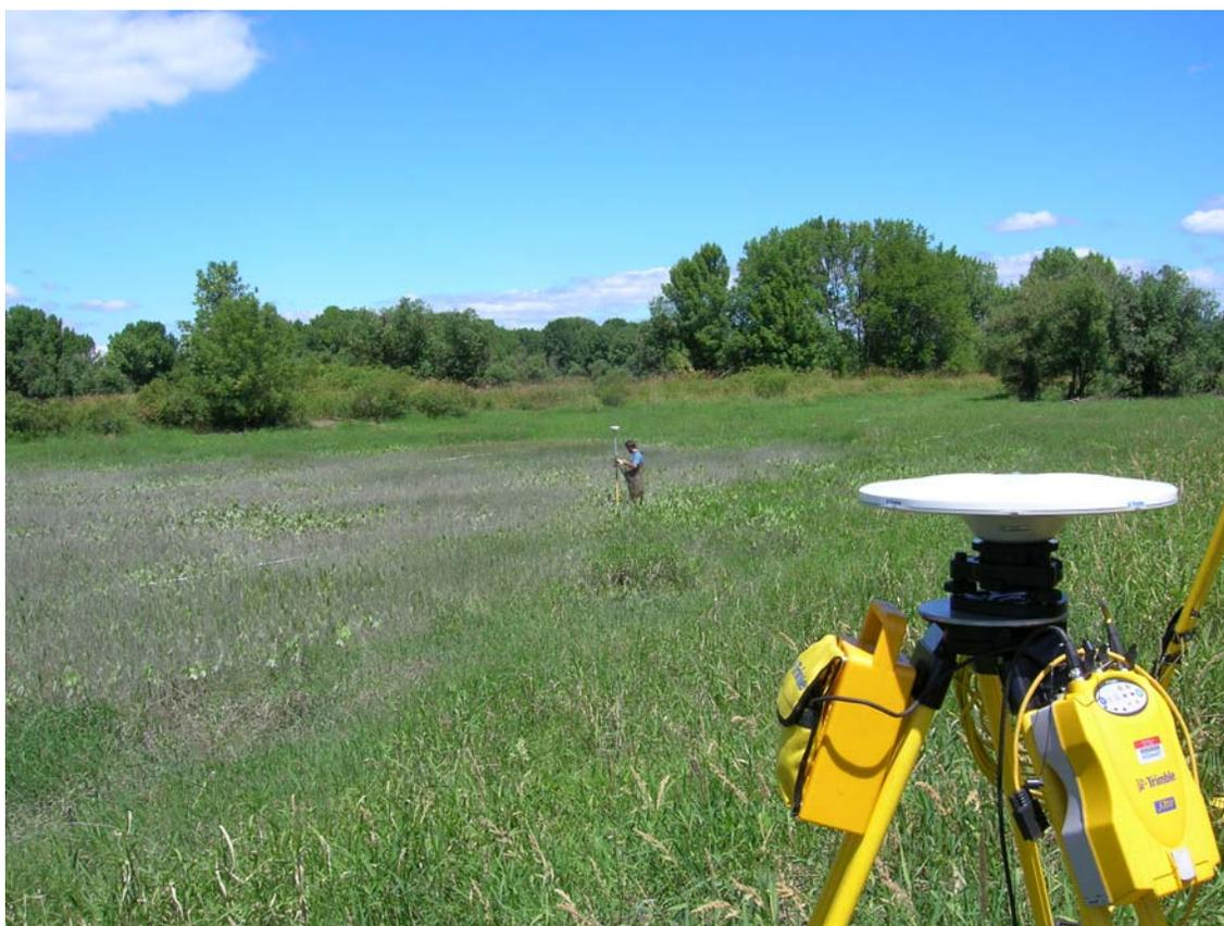
**Figure 27: Grid survey showing RTK base station and rover (in the distance).**
