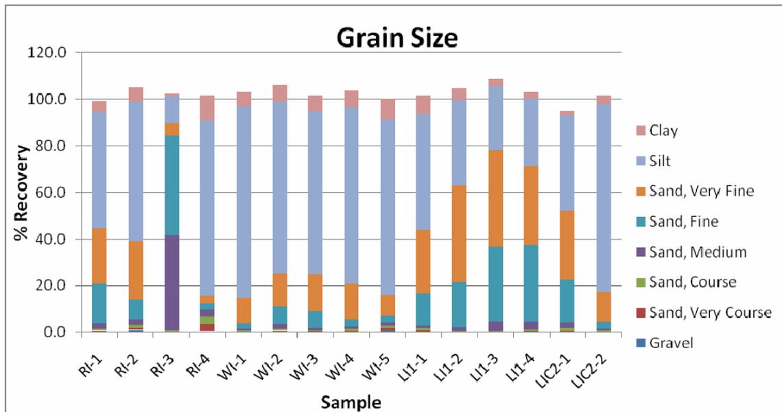
Figure 19: Grain size distribution in the sediment samples from 2009 monitoring sites in Reach C.
