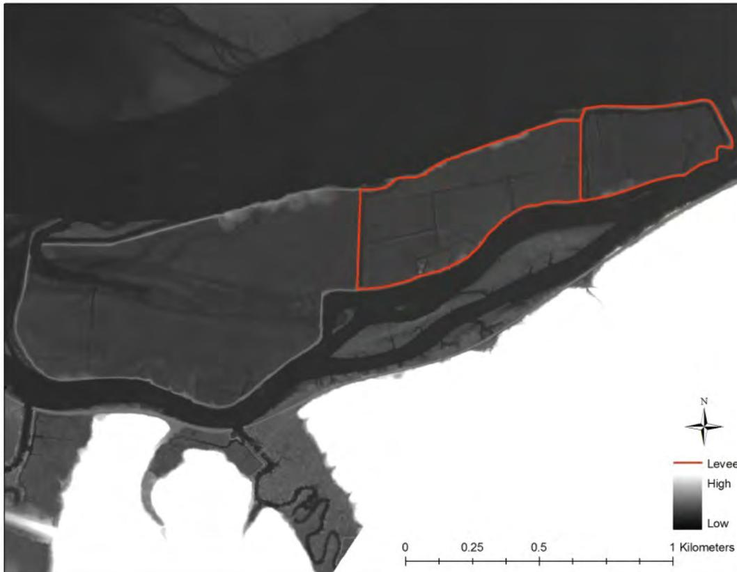
**Figure 4: Levee delineation (red line) at Svenson Island. A relic levee around the west end of the island is evident from the Lidar; however, a gap at the NW corner of the island allows for regular tidal inundation of the area.**
