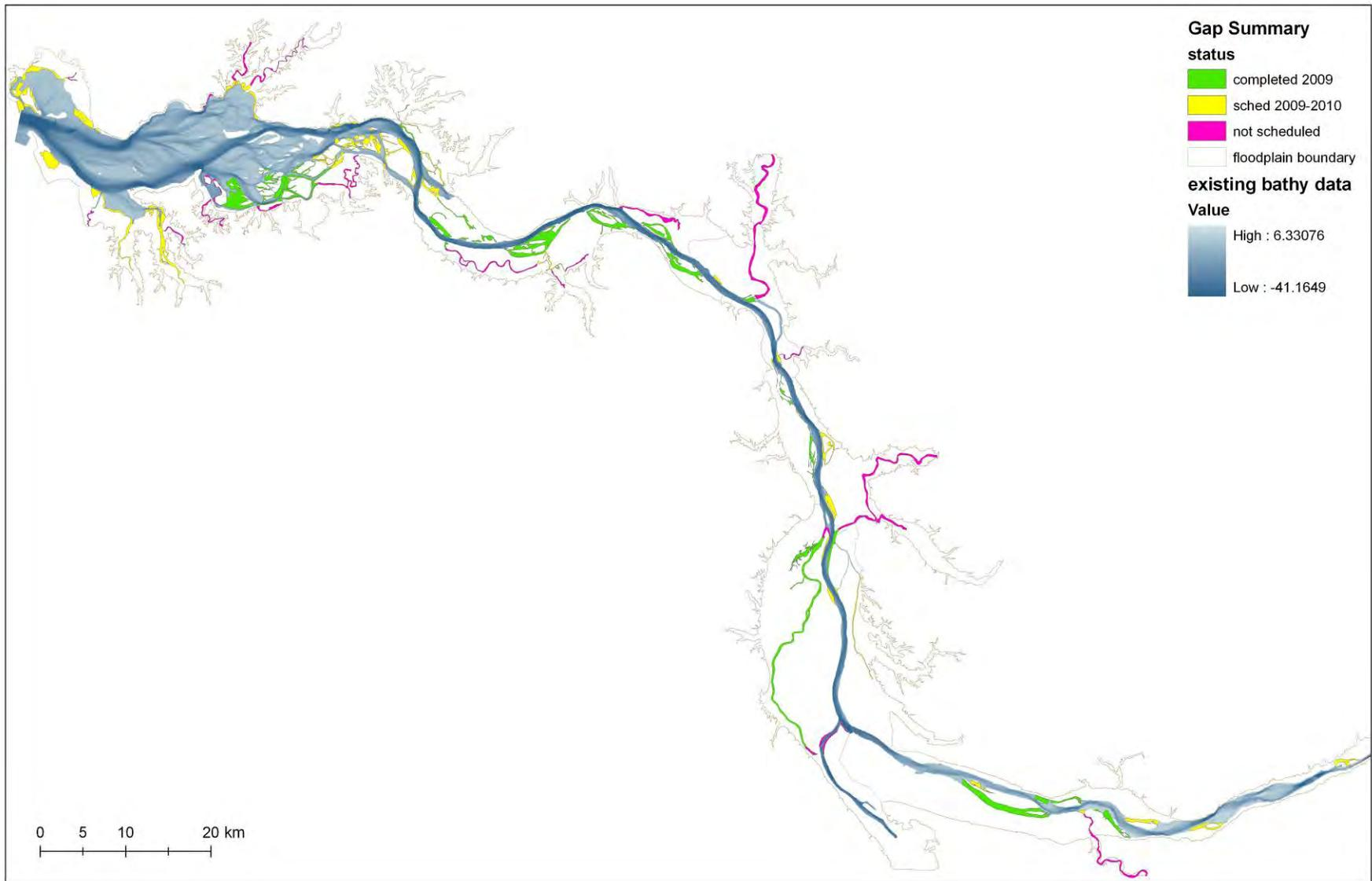
**Figure 10: Map of LCRE showing bathymetry data collected in 2009 (green), bathymetry scheduled for collection in 2009-2010 (yellow), and remaining bathymetry gaps not scheduled for collection (pink).**
