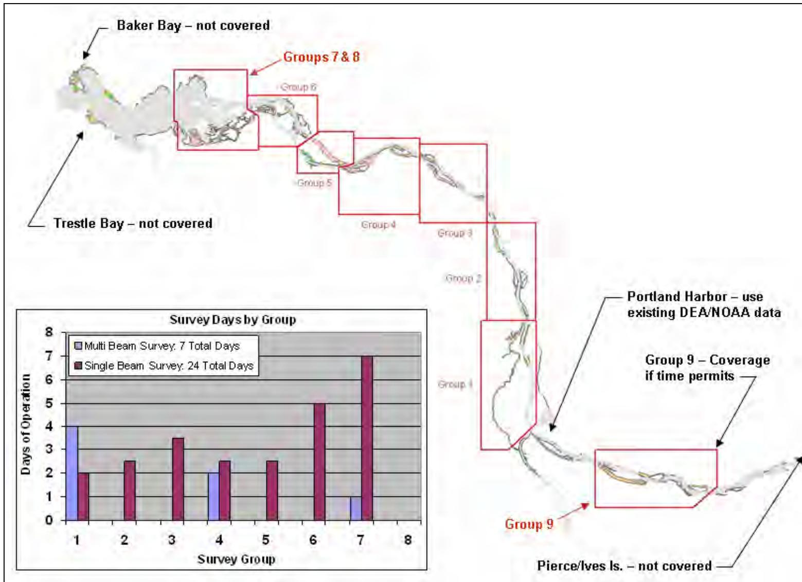
Figure 9: Bathymetry survey plan showing LCRE divided into 9 collection groups. Inset table shows days of survey by group. In 2009, high and medium gaps were filled in Groups 1-5 and 9. In 2010, gaps in Groups 2, 6, 7/8, and 9 will be targeted for collection.
