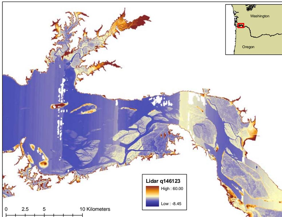
**Figure 4; Lidar bare earth elevation DEM, including the water surface elevation values that varied with the tide level during the survey flights.**
