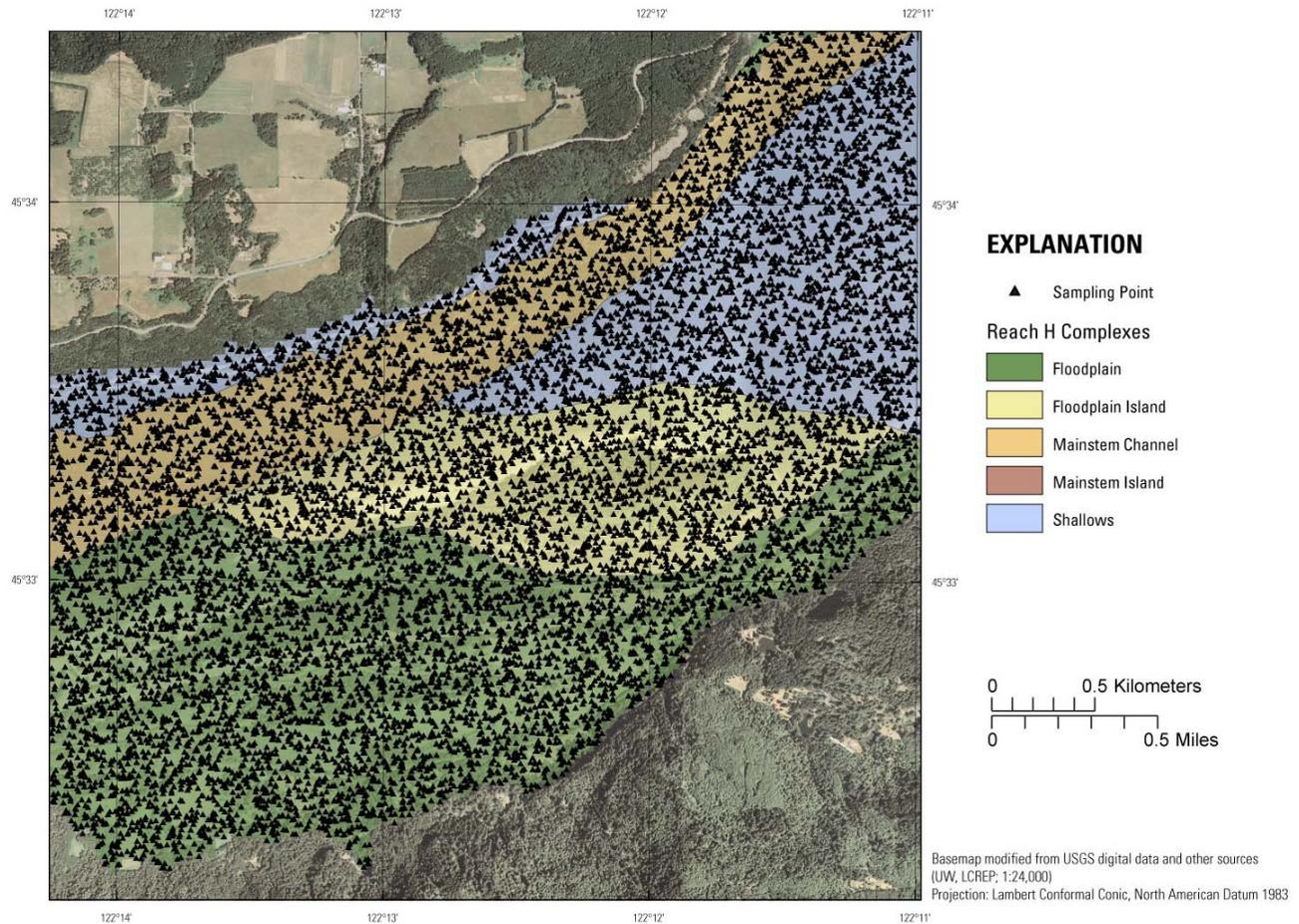
**Figure 5: Portion of Reach H complexes and overlay of master point grid (denoted by black triangles), illustrating the high density of potential sampling sites in a reach and across complexes.**
