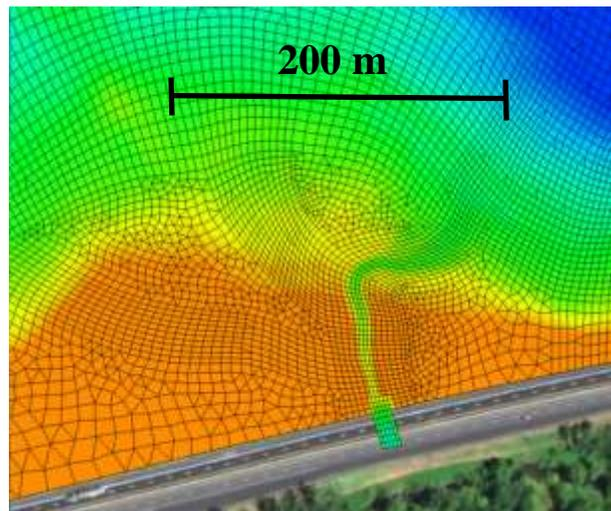
**Figure 33.** Tuflow model mesh generated for cold-water plume analysis. Top: mesh extent in lower Columbia River Gorge; bottom left: mesh detail at Bridal Veil Cr. confluence; bottom right: mesh detail at Multnomah/ Wahkeena Cr. confluence. The same elevation scale applies to all images.
