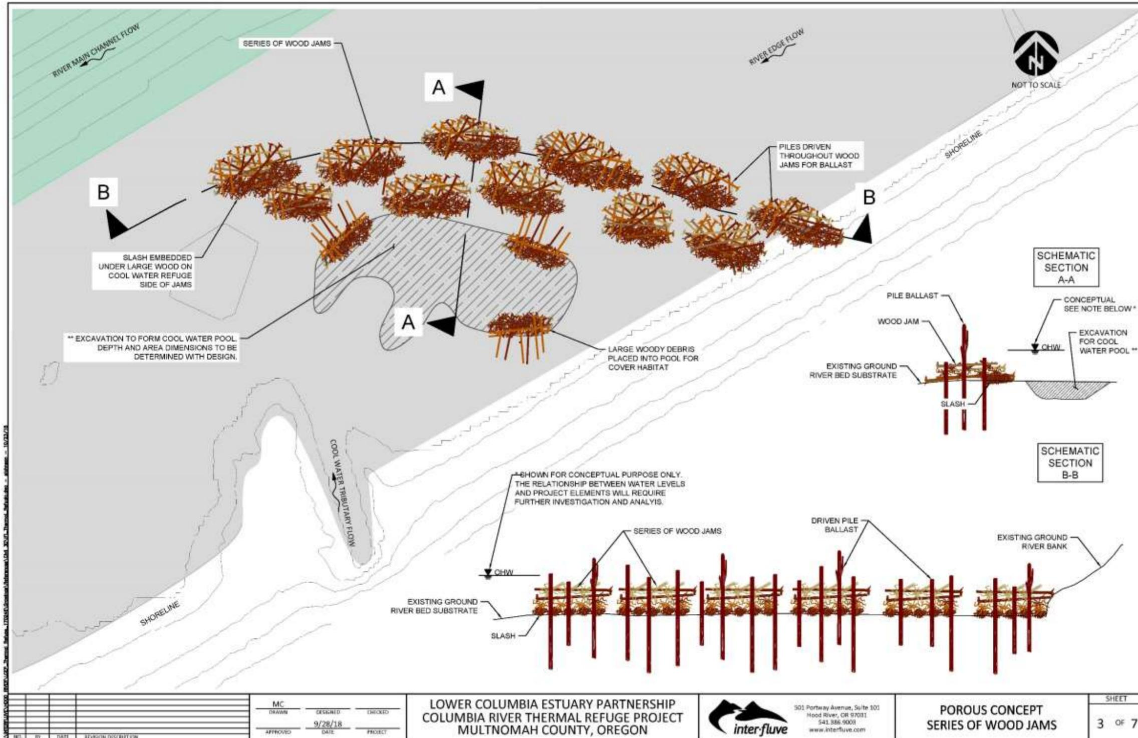
Figure B-15: Conceptual approach for thermal refuge enhancement structure placement at selected tributary confluences (Study Phase 3). Sketch 3 of 7.
