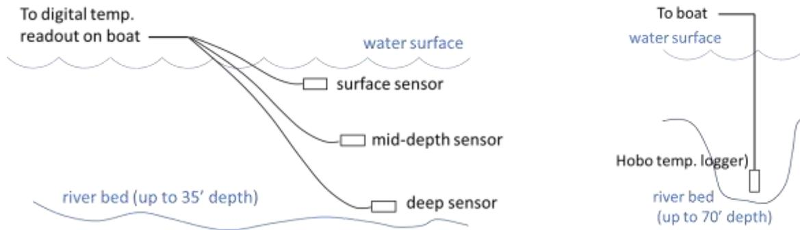
**Figure 19.** Schematics of temperature sensor deployment for Phase 2 mainstem Columbia and downstream tributary temperature monitoring. Left: custom sensors used for continuous monitoring of water column up to 35’ depth. Right: HOBO data logger deployment at deep water locations.
