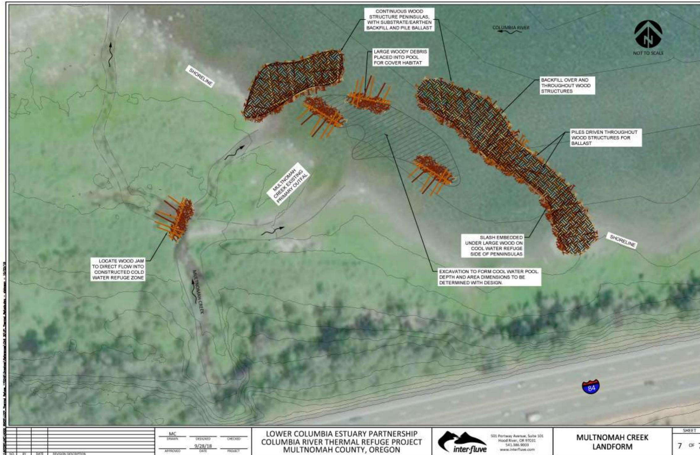
Figure B-15: Conceptual approach for thermal refuge enhancement structure placement at selected tributary confluences (Study Phase 3). Sketch 7 of 7.
