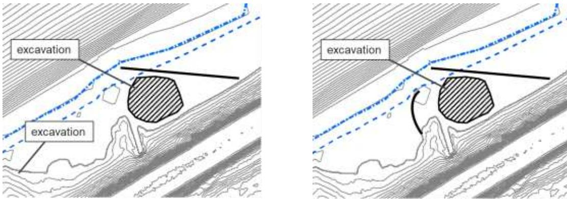
**Figure 41.** Scenario 3 (left) and 4 (right) structure placements for the Horsetail/Oneonta confluence, with excavation to 2-meter depth.
