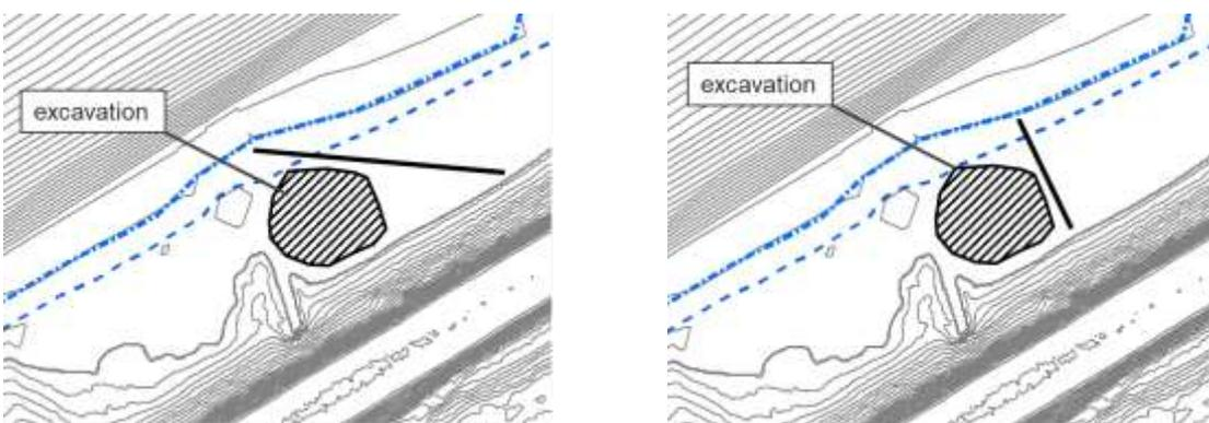
**Figure 40.** Scenario 1 (left) and 2 (right) structure placements for the Horsetail/Oneonta confluence, with excavation to 2-meter depth.
