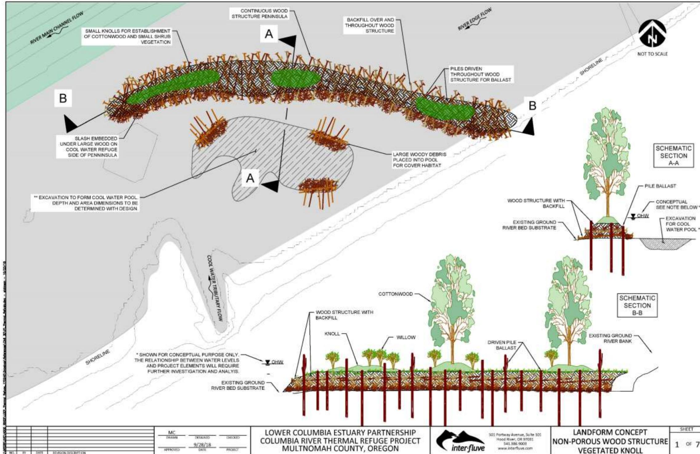
Figure B-15: Conceptual approach for thermal refuge enhancement structure placement at selected tributary confluences (Study Phase 3). Sketch 1 of 7.
