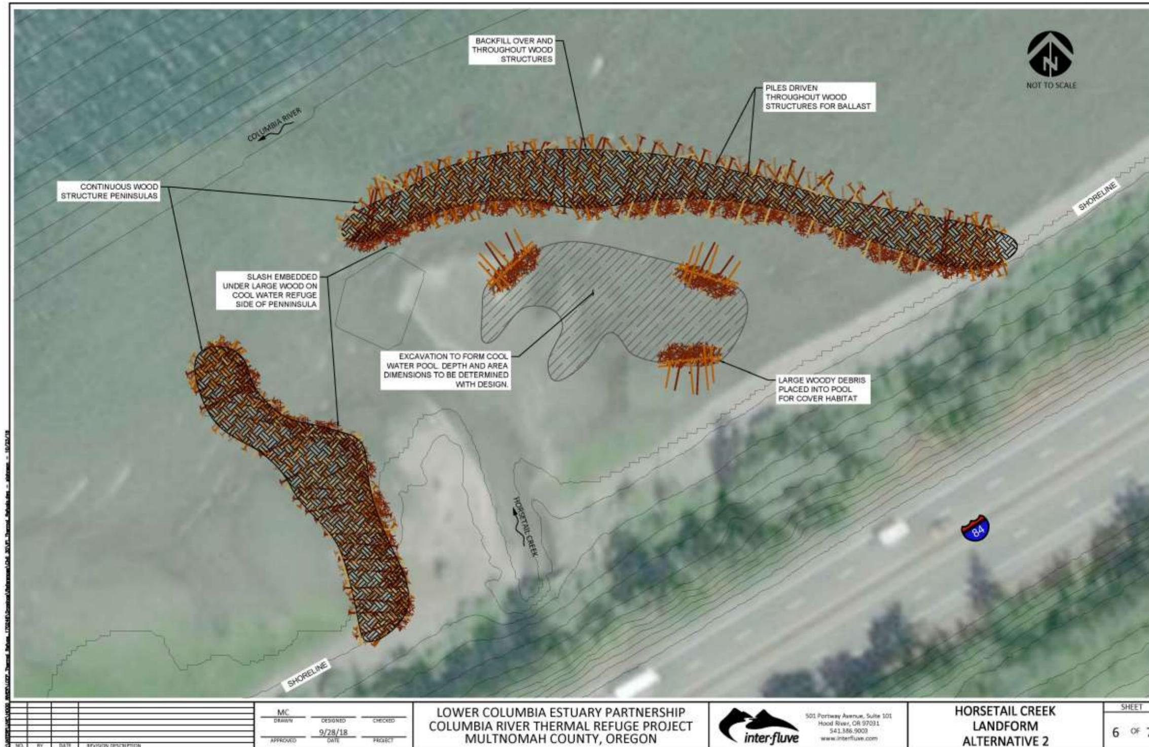
Figure B-15: Conceptual approach for thermal refuge enhancement structure placement at selected tributary confluences (Study Phase 3). Sketch 6 of 7.
