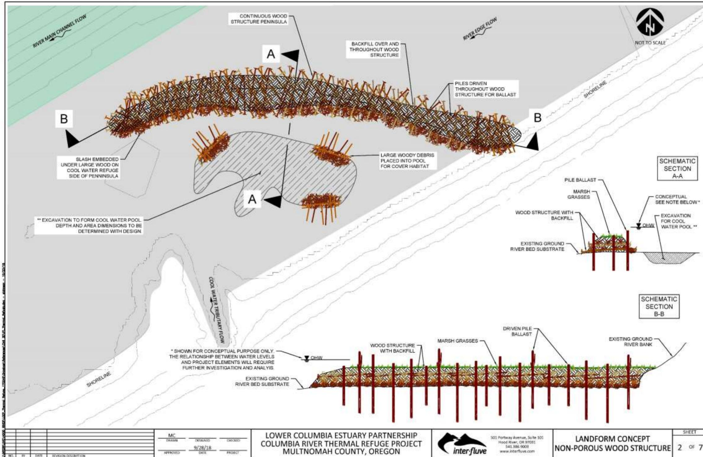
Figure B-15: Conceptual approach for thermal refuge enhancement structure placement at selected tributary confluences (Study Phase 3). Sketch 2 of 7.
