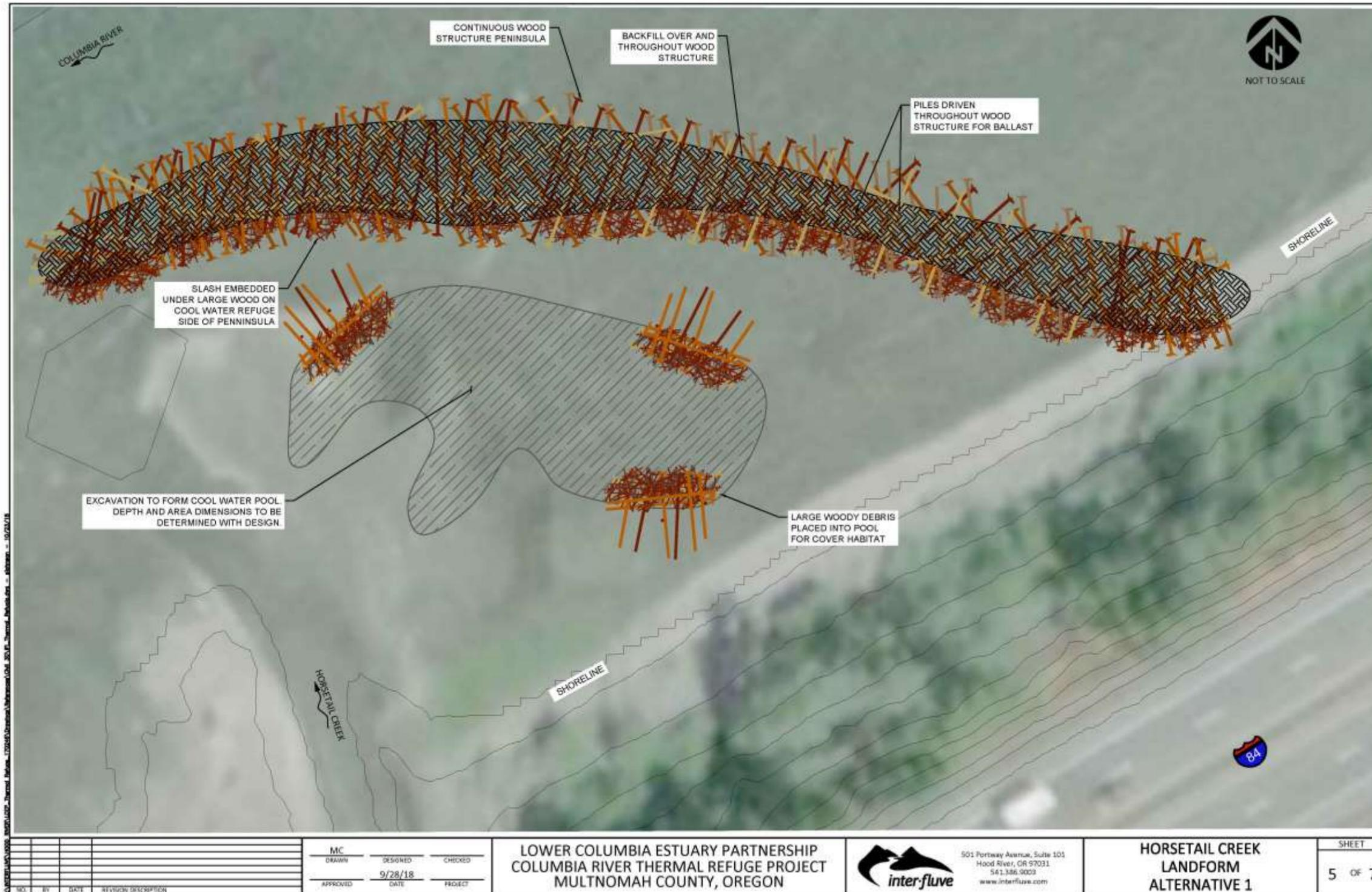
Figure B-15: Conceptual approach for thermal refuge enhancement structure placement at selected tributary confluences (Study Phase 3). Sketch 5 of 7.
