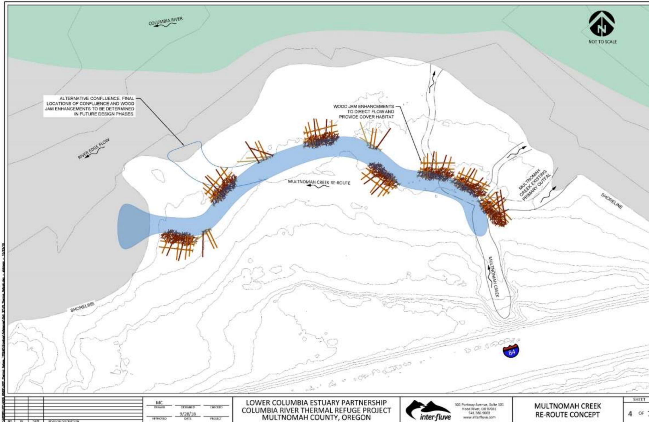
Figure B-15: Conceptual approach for thermal refuge enhancement structure placement at selected tributary confluences (Study Phase 3). Sketch 4 of 7.
