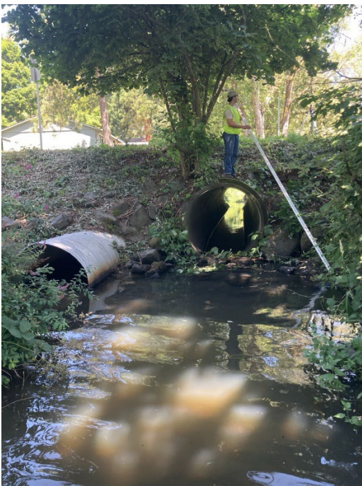
University of Portland summer student intern assisting with fish passage assessment of a culvert along Weaver Creek in Battle Ground, WA.
