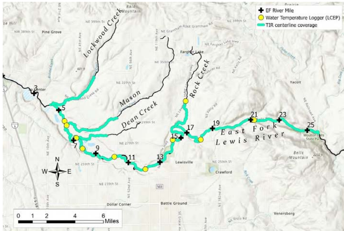
Figure 6. Extent of coverage (shown as blue area) for the TIR airborne survey, including the lower EFLR from RM 4–25 and four primary tributaries. Locations of installed data loggers used for image calibration are also shown.
