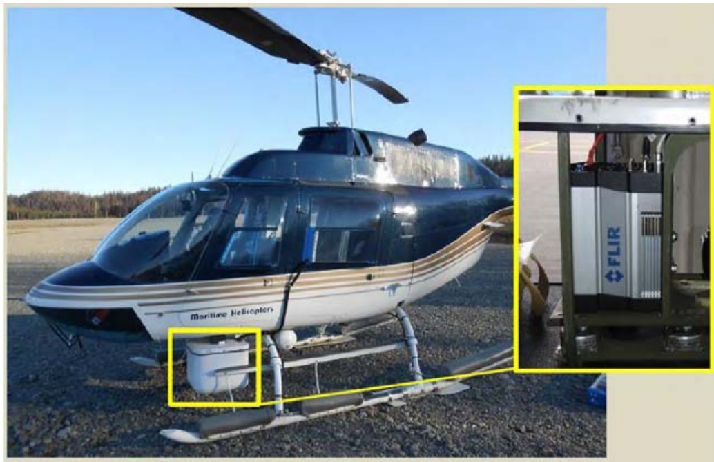
Figure 1: Sensor and aircraft setup (similar to the setup used for the project)
