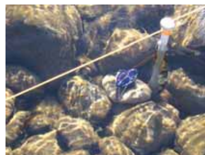
Temperature logger installed to monitor a cold water habitat site
