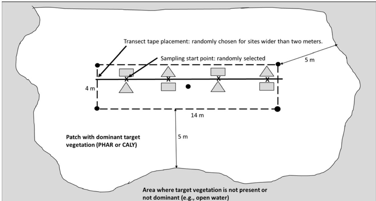
**Figure 2. Simplified diagram of sampling setup at a site (site dimensions are an example only). The solid black line represents the transect tape. Gray rectangles = fallout traps and gray triangles = emergence traps. X's indicate the randomly selected sampling locations and the location of benthic cores. Filled black circles represent the PVC poles placed as markers at the corner and center of each site.**
