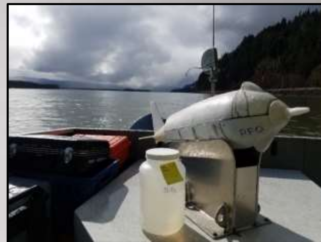
D-96 depth integrated sediment sampler on the Columbia River, photo credit: P. Diaz
