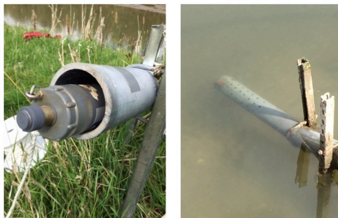
Figure 6. Images are showing deployment of water quality monitors (YSI sondes) at study sites.
