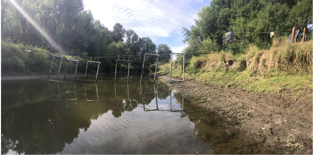
Figure 9. Image of the new PIT detection system at Campbell Slough, installed February 2018.
