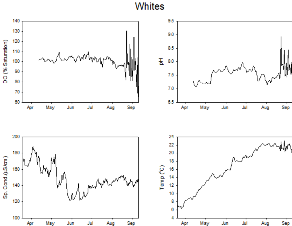
Figure 20. Time series of daily averaged measurements of water quality parameters made at Whites Island, 2019.
