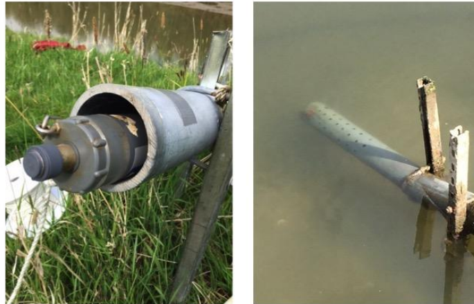
Figure 7. Images are showing deployment of water quality monitors (YSI sondes) at study sites.
