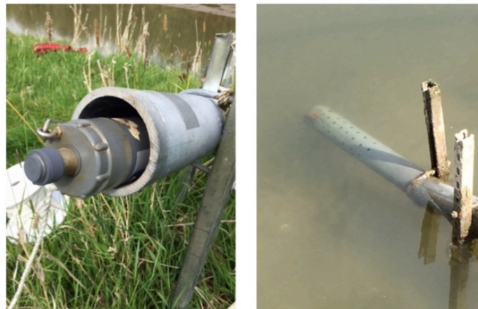
Figure 5. Images showing deployment of water quality monitors (YSI sondes) at study sites.
