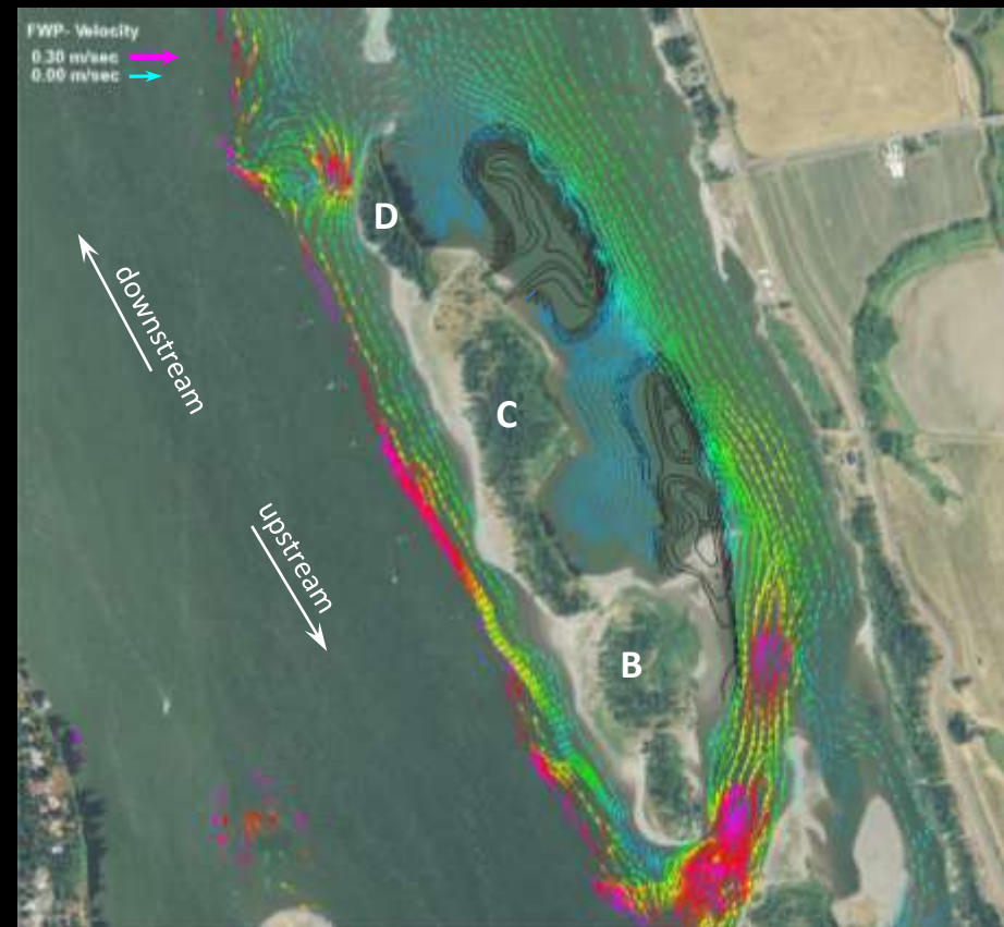
RIGHT. FWP River Currents – Ebb Tide during LOW riverine flow. Both figure H3a and H3b are “snapshots” of river current vectors simulated by AdH model for 1400 on 13 JUL 1997 (model TS=2486 hrs).
