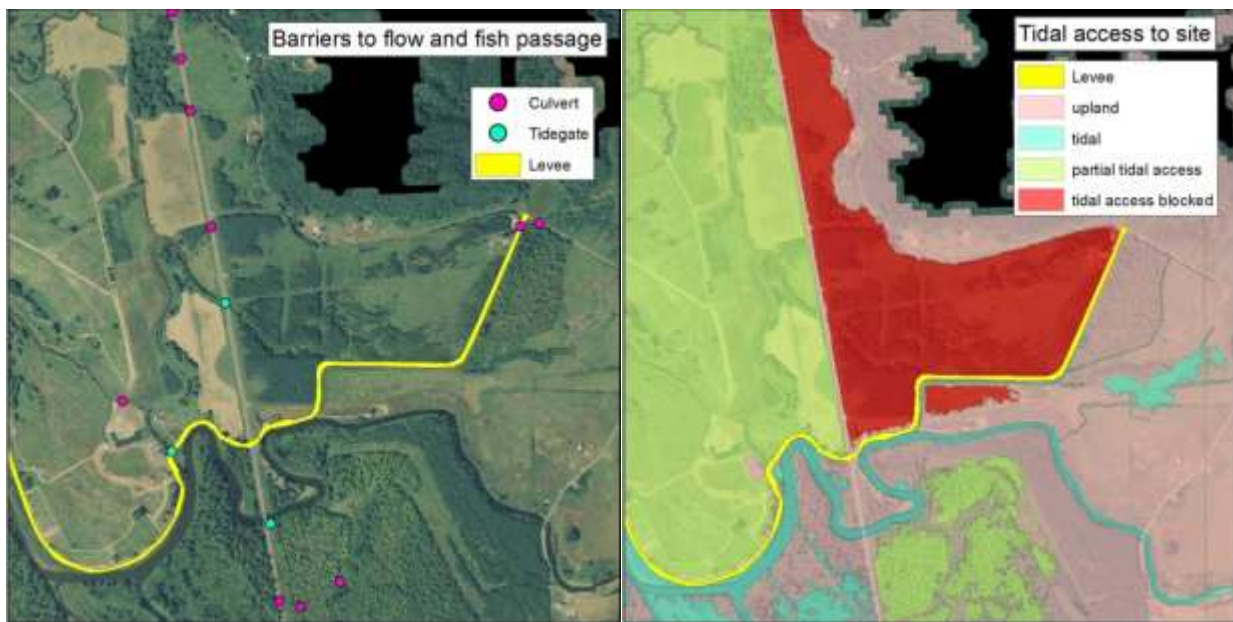
Figure 10. Example of applying landscape assessment tools to a sample parcel, with a levee restricting flow and fish access. Fish passage barrier inventory dataset overlain on aerial image of several parcels, with the tidally impaired dataset shown.
