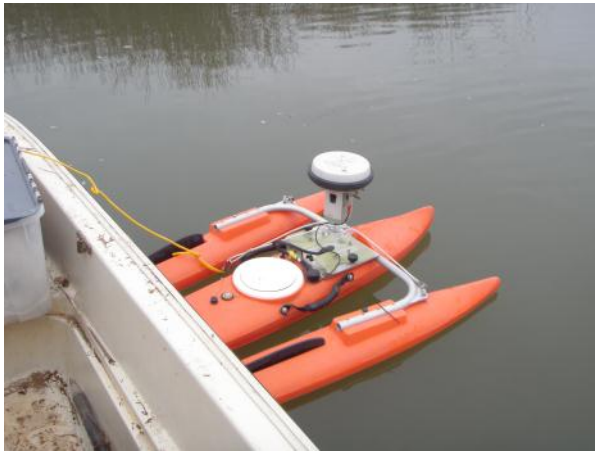
Acoustic Doppler Current Profile (ADCP) used to measure channel bathymetry and currents flow. April 12, 2012.
