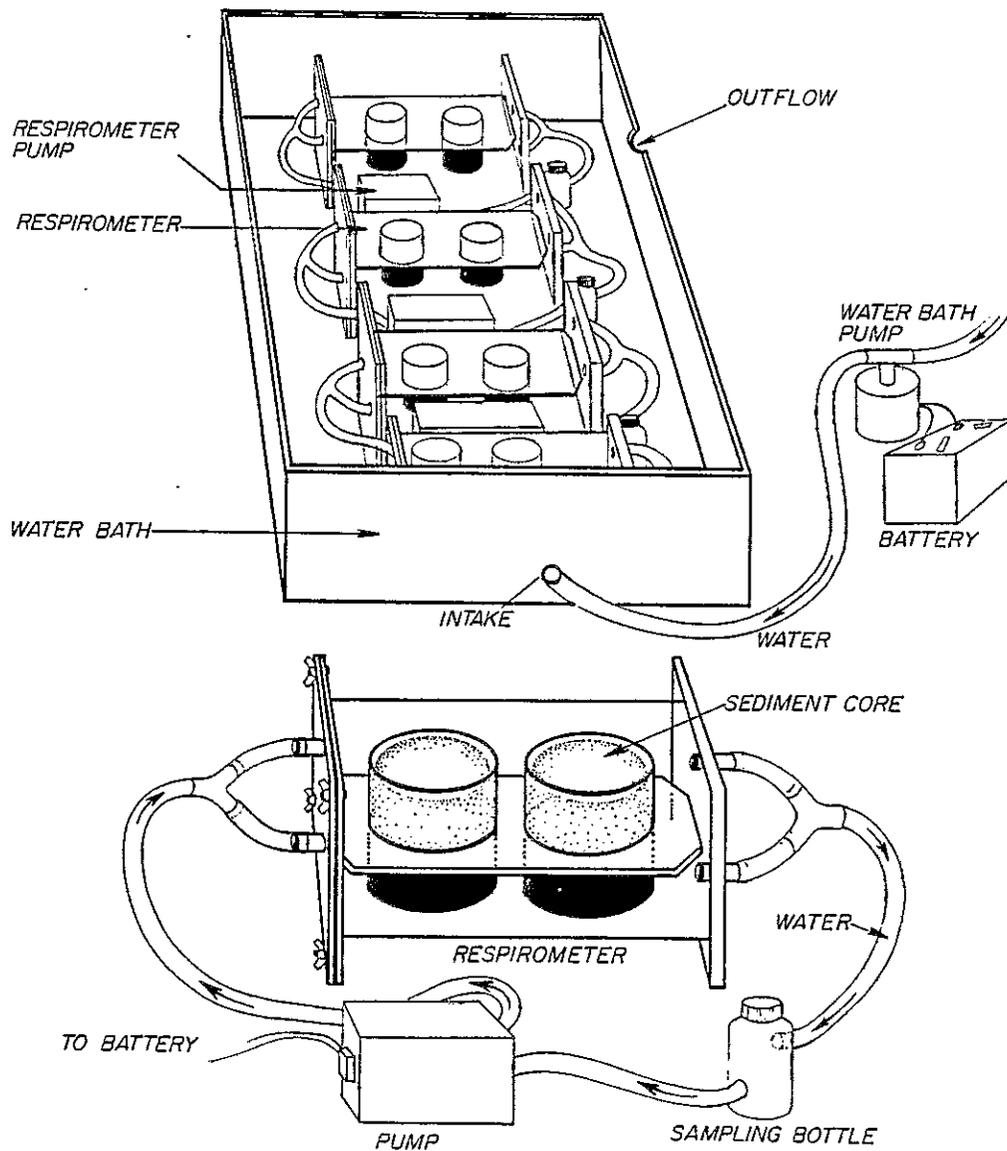
Figure 4. Diagram of the apparatus used to measure benthic primary production in the Columbia River Estuary.
