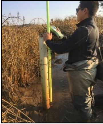
Figure 8. Surveying data logger elevation from crossbar.
