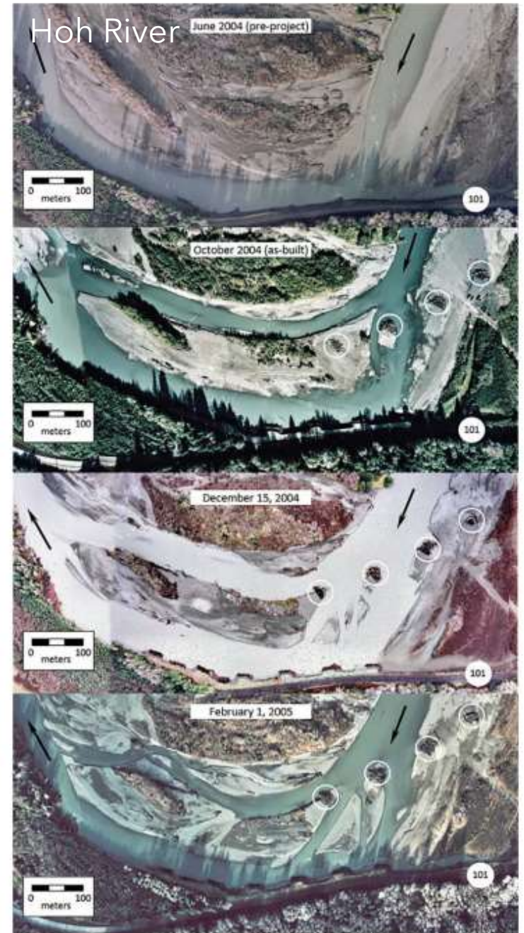
Fig. 2 Time sequence photos of pre-and post-project conditions for ELJs re-directing flows on the Hoh River, Jefferson County, WA.
